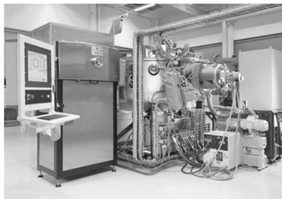
Fig. 10 DC magnetron sputtering system NESSY
